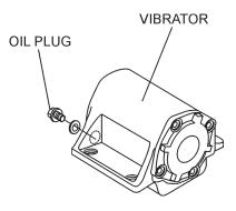
Figure 5. Vibrator Oil Plug
